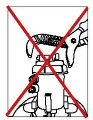
Clamping the plastic housing in a vice and attempting to loosen the filter fastening ring with a large pair of metal-jawed grips is highly likely to result in damage.
