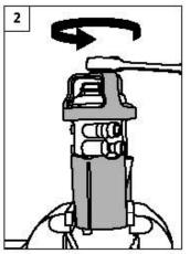
Clamp part 'A' into a vice. Remove Using a 1/2" drive ratchet simply undo the fastening ring by
