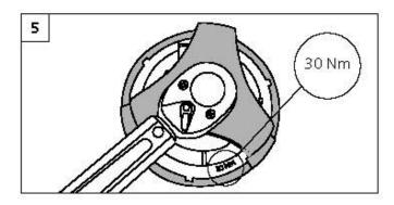
Tighten the fastening ring to 30Nm, then refit the housing to the vehicle and reconnect all fuel pipes and electrical connectors. Start the engine and check for leaks.
