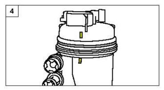
Replace the rubber seal between the two sections of the housing with the one supplied with the new filter. Refit the upper section to the housing by aligning the yellow/green markers.
