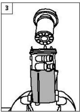
Extract the upper section of the filter housing and replace the fuel filter element taking care not to touch the filter paper on the new element.
