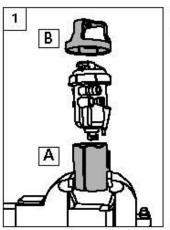
fuel filter housing from vehicle, taking care to remove all pipes turning part 'B' anti-clockwise. and all electrical connectors. Place the filter housing into part 'A' and locate part 'B' onto the top of the housing, aligning the six slots of the tool with the filter housing fastening ring.
